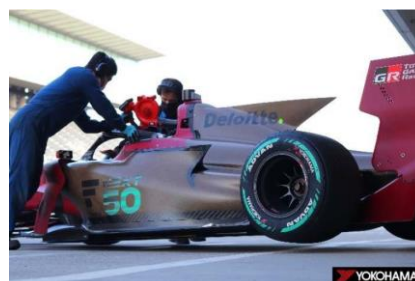
Development car with lower downforce than SF19 cars
