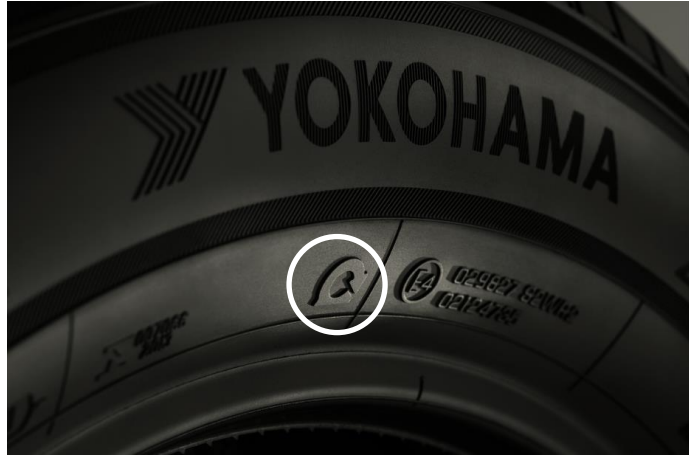
Mark on BluEarth-XT AE61 Z·P·S indicating conformity with the EMT standard
