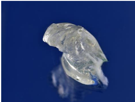
Butadiene rubber generated using the world's first butadiene produced by fermentative production
