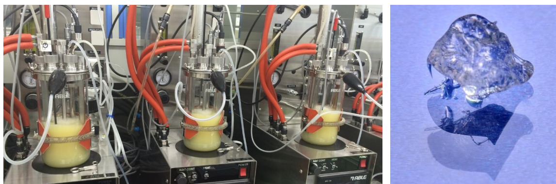
In-cell (in vivo) synthesis of isoprene (left) and polyisoprene rubber polymerized using the new technology
