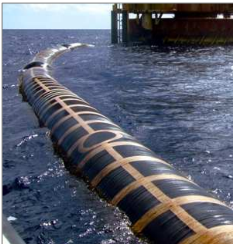
A Yokohama Rubber Seaflex hose in action during a crude oil transfer operation
