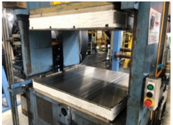
[After Insulating Paint Application]
