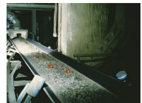
Highly heat-resistant conveyor belt
