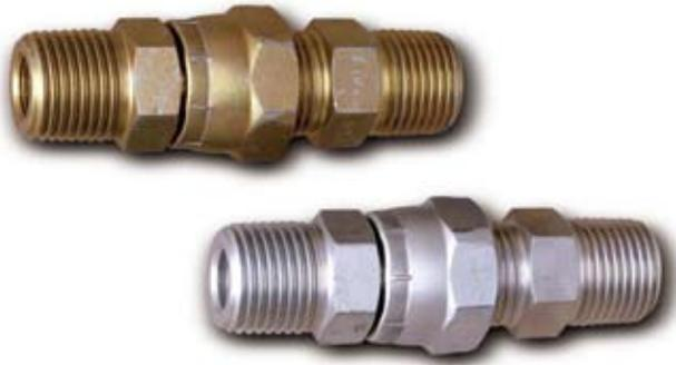
*Yokohama has replaced hexavalent chromium (upper photo) with trivalent chromium (lower photo) as a coating material for zinc-plated hose fittings. The change is in response to medical and environmental concerns about hexavalent chromium. Yokohama began the changeover in June 2007 and has largely completed the transition to the more-benign material.*
