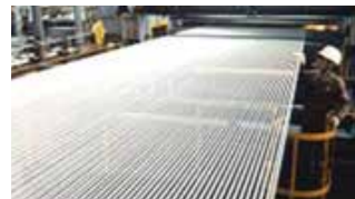
In 1970, installed German-made equipment for producing a 3.2-meter wide steel cord conveyor belt at the Hiratsuka Factory.
