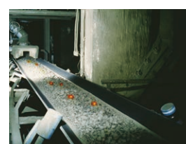
Highly heat-resistant conveyor belt
