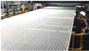
In 1970, installed German-made equipment for producing a 3.2-meter wide steel cord conveyor belt at the Hiratsuka Factory.
