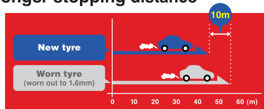
At the same speed (80km/h) and from the same braking point, there is a difference of 10 metres! *Japan Automobile Tire Manufacturers Association
