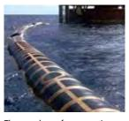
These are hoses for connecting tankers anchored offshore and onshore facilities and transporting crude oil. Since the hoses are installed in the special environment of the ocean, abundant experience and advanced technical capabilities are required for design that fulfills durability requirements in order to withstand severe storms such as typhoons. There are only a very few companies around the world capable of designing and manufacturing marine hoses.
