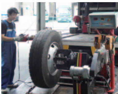
■ Replacement, removal, air adjustment work of tires using a machine for tire replacement work for trucks and buses.
