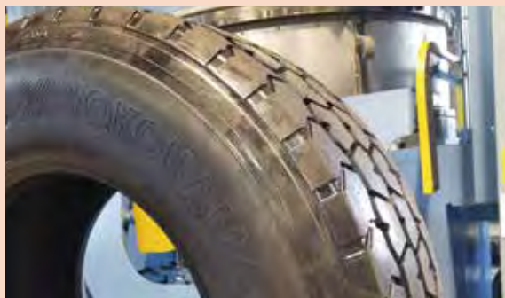
Wide-based size retread tires subject to rigorous evaluation by Yokohama Rubber after the prototype was made at the Saitama Office
